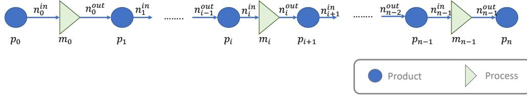
Figure 1: A sample production graph, with manufacturing processes  $m$  and products  $p$ . Numbers (denoted by  $n$ ) on edges indicate the quantity consumed or produced by the corresponding manufacturing process.
